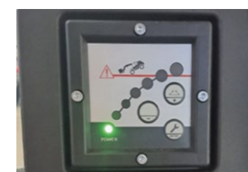
Anti-rollover system for 5" displays.
