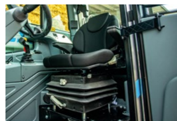
Seat with air suspension as an option for both ranges.
