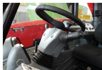
Adjustable steering column, via side lever.
