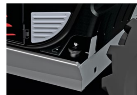
Fuel tank positioned under the cab for excellent protection (standard version).
