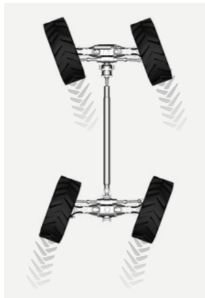
Concentric: guarantees a narrower manoeuvring radius.
