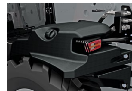
Diesel tank positioned behind the cab for the Low Cab variant of FS Compact.
