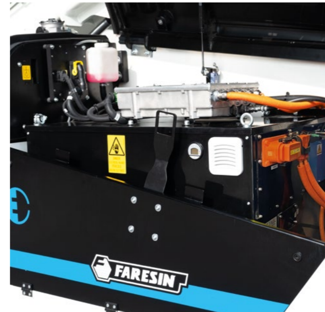
435 V lithium battery pack available with a power of 105 Ah.
