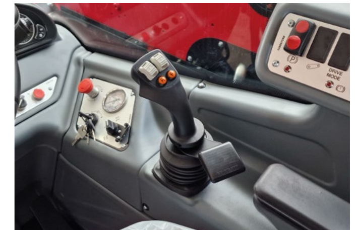
Standard Electro-proportional Mechanical joystick for CLASSIC versions.
