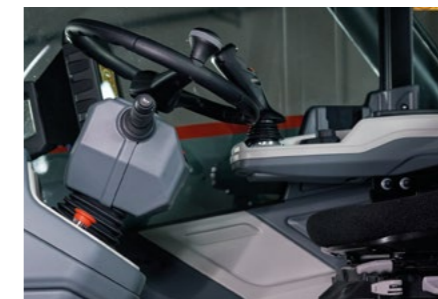
Steering column tiltable via side lever.
