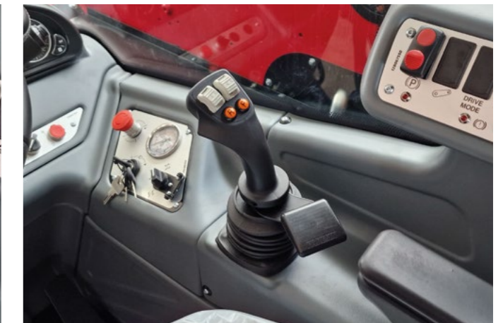
Standard Electro-proportional Mechanical joystick for CLASSIC versions.
