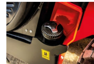
The diesel tank is equipped with a lockable cap, positioned in the lower part of the cab to guarantee excellent protection.
