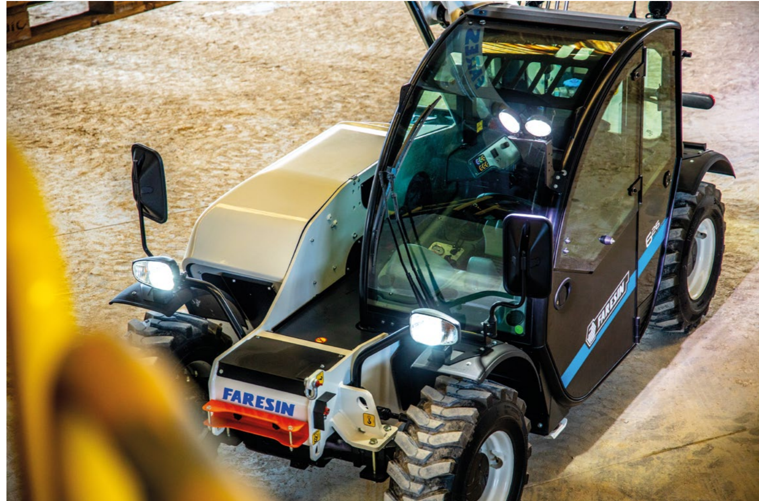
Cab and Electro-proportional Mechanical joystick as standard on 6.26 Small Range Full Electric.
