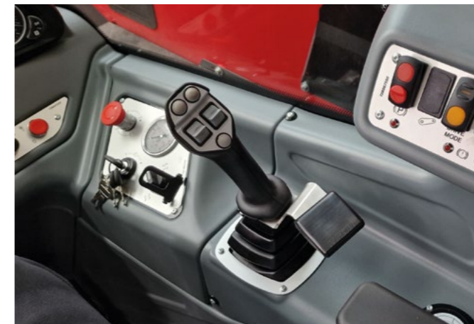
Electro-proportional hydraulic multi-function joystick available in versions HLS and VPSe.
