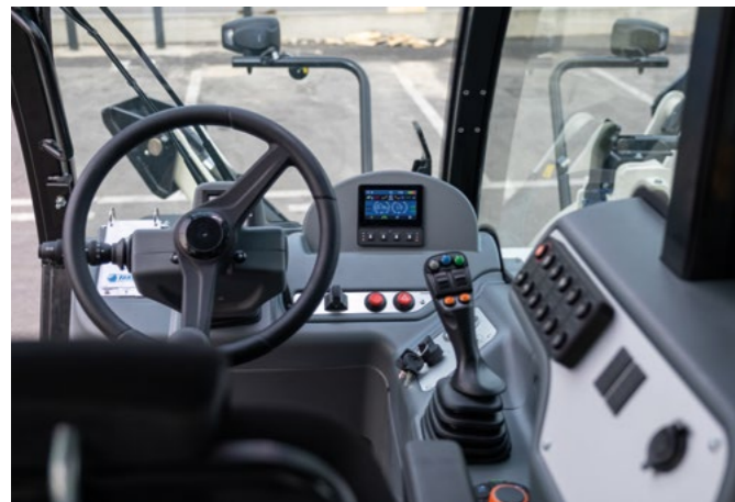
Cab and electro-proportional hydraulic joystick as standard on Big Range Full Electric.
