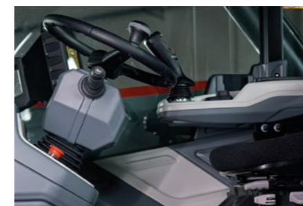
Steering column tiltable via side lever.
