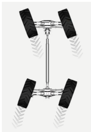
Concentric: guarantees a narrower manoeuvring radius.
