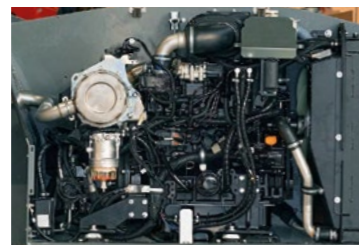
51.7 kW Yanmar engine, available in the 6.26 Small Range.
