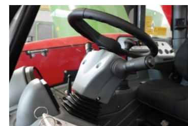
Adjustable steering column, via side lever.
