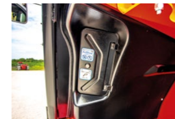
The AdBlue tank is protected by a plastic casing, located at the rear of the cab.
